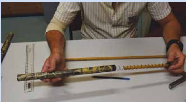
Figure 2. Place the dowel in the spring and return it to the magazine cylinder.
