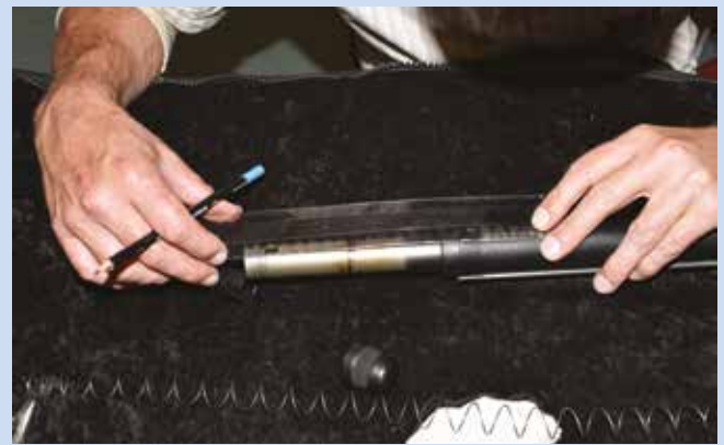
Figure 3, For the semi-auto measure 159mm from the breech end and place a mark
