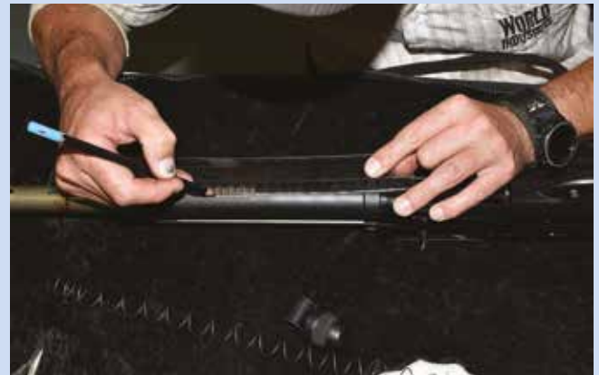
Figure 4. Measure from the mark to the end of the magazine or if there is an end stopper to this point. This is how long your dowel needs to be.
